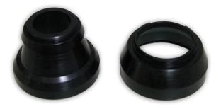
7) A CCD camera will attach to the HyperStar using T-threads. Most cameras have a 1.25" or 2" nosepiece that must be removed to allow the HyperStar to thread into the T-threads. SLR cameras attach using a standard bayonet mount identical to a camera lens mount. Locate the mark on the HyperStar adapter and line this up with the mark on the camera body as you would a normal lens.
