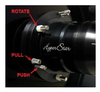
**Note:** Do not overtighten the collimation screws, as this will cause the HyperStar lens to be difficult to remove from the telescope.
